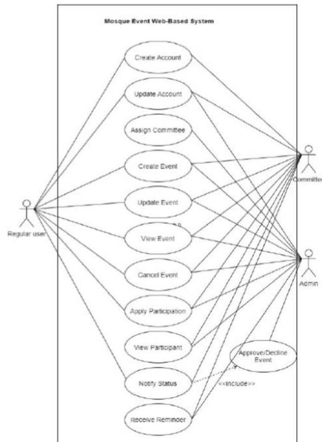
Figure 1: Use Case Diagram for Mosque Event Web-based System
