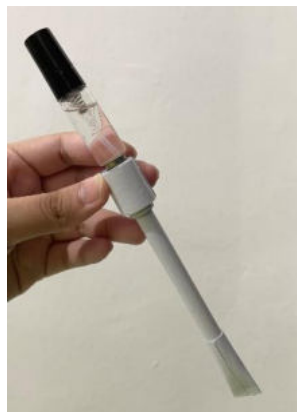
Figure 1: MisTic covered with pen cap and attached to a spray vial with permanent magnets
