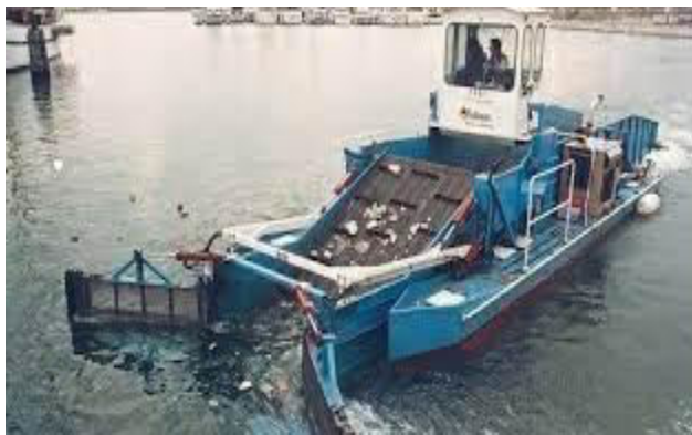
Figures 1 and 2: A trash skimmer boat for large scale cleaning
