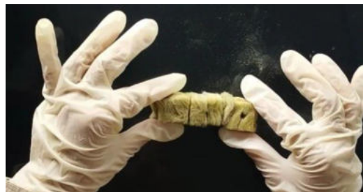
Figure 1: On the black fabric, rockwool leaves a fine dust mark. The fine dust is extremely hazardous to one's health.
