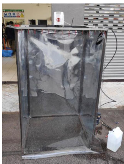
Figure 3: Finalized fabricated product Full-Body Sanitization Machine
