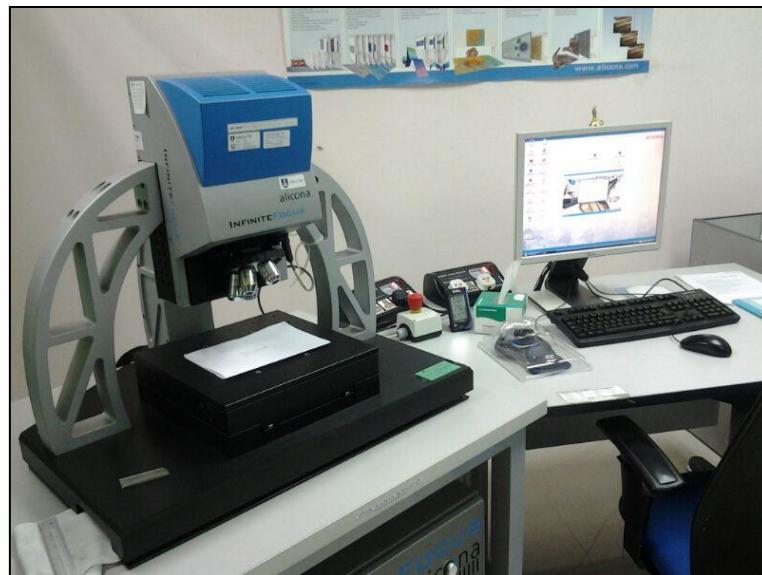
Figure 1: ALICONA Infinite-Focus optical 3D surface metrology apparatus
