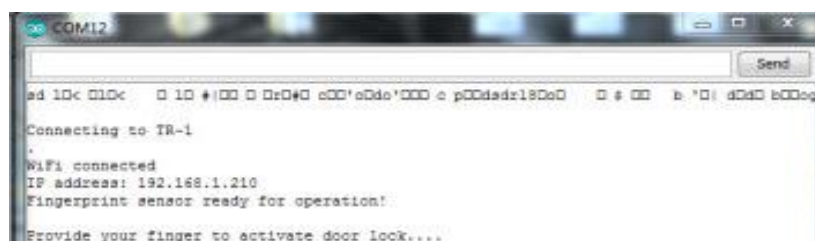
Figure 5: Connected Wi-Fi Display in Arduino COM Serial Monitor
